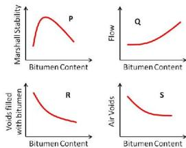
Theoretically plausible correct graphs according to the 'Marshall mixture design output are
