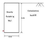
The minimum weight of the wall (expressed in kN per m length) required to prevent it from overturning about its toe (Point P) is
