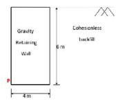
The minimum weight of the wall (expressed in kN per m length) required to prevent it from overturning about its toe (Point P) is
